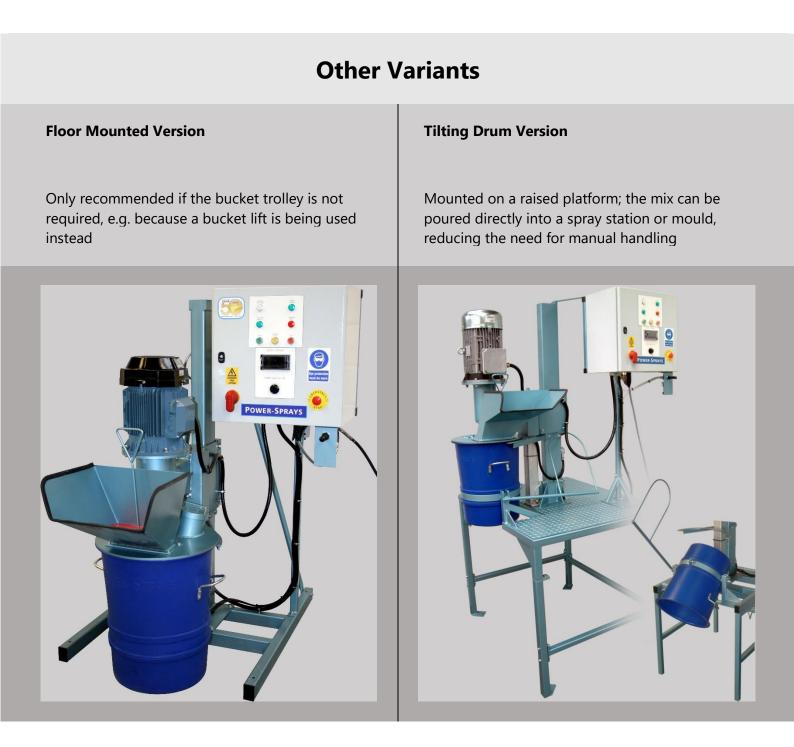
The GRC 125 Combination mixer is the first mixer that can produce spray grade GRC slurry and also premix GRC without compromise. The unit has a generous 65 litres capacity, which easily accommodates 125kg of material i.e. a mix based on 50kg of cement and 50kg of sand. It works equally well with a mix based on a 25kg bag of cement.
