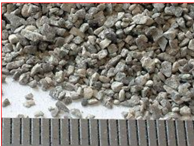
BAD – Angular particles, poor distribution of sizes
