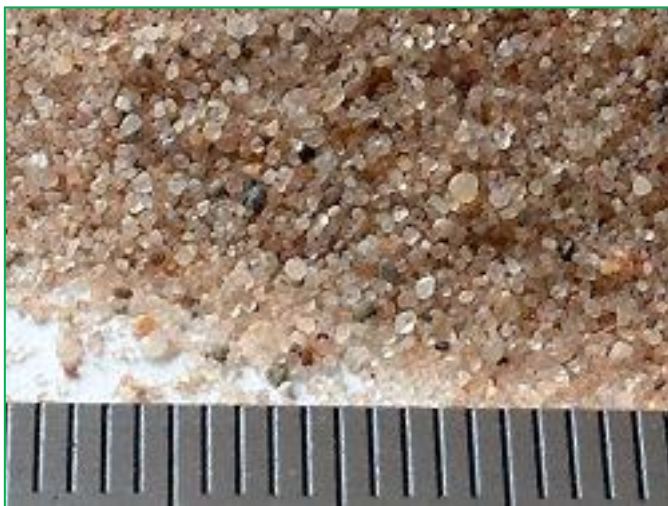
GOOD – Rounded particles, good distribution of sizes
