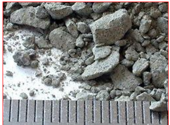
BAD – Angular particles, larger than 1.2mm
