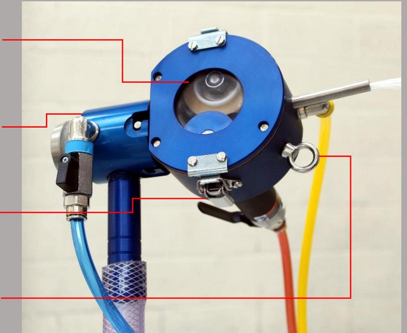
The new Power-Sprays' Concentric Spray Head is designed for the efficient spray application of Glass fibre Reinforced Concrete (GRC). It is to be used with the new improved boom fitted to Power-Sprays spray stations.
